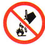
禁止用水灭火 NO EXTINGUISHING WITH WATER
